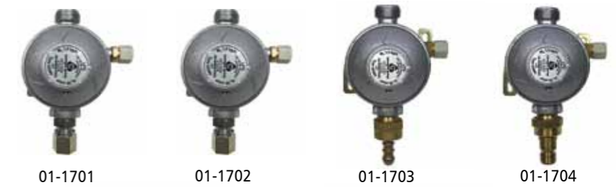
The Clesse 30mbar low pressure regulator is suitable for use with either propane or butane or European LPG on installations in mobile touring leisure accommodation vehicles, for bulkhead mounting into vented cylinder compartments
